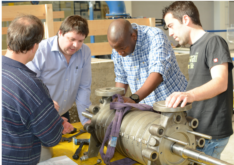
Installation of a multi-stage pump on the pump assembly module at Graz University of Technology.
